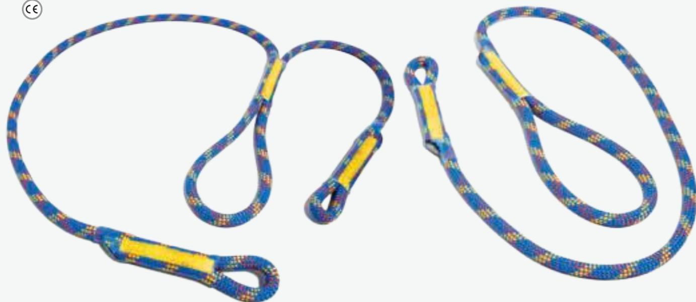
DynaProt 10, the dynamic sling, is made of a dynamic rope and is therefore capable of absorbing the energy of a dynamic fall and to dampen this fall thanks to its elongation. DynaProt 10 has been tested with fall factors 1 and 2. It is able to arrest nine falls with a fall factor of 2. Even with a fall factor of 2, the impact force is lower than the maximum force permitted by EN 892.
