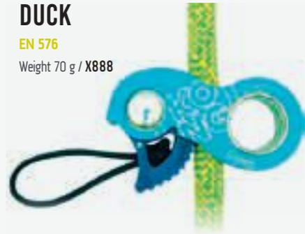
Duck - a new rope clamp/positioner made by Kong, designed for ropes with diameters between 8 and 13 mm. The first and only device that may be used also with 10 to 15 mm wide flat and tubular slings. Due to its small dimensions, it is possible to use Duck with one hand only, the large diameter enables the karabiner to rotate. Intended for ascending activities, daisy chain positioning, self-belaying.
